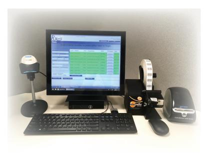
The RxAWS (Auxiliary Workstation) complements the RxSafe 1800™ and RxSafe 900™ by adding one or more workstations for checking in inventory, putting away remote stock, and filling prescriptions from remote stock. Additionally, all of the standard features of the RxSafe system, including reports, can be accessed from the RxAWS.
